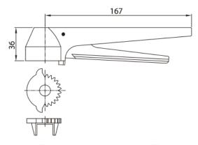
12-Position Gripper Handle, made from Stainless Steel and Nylon.
